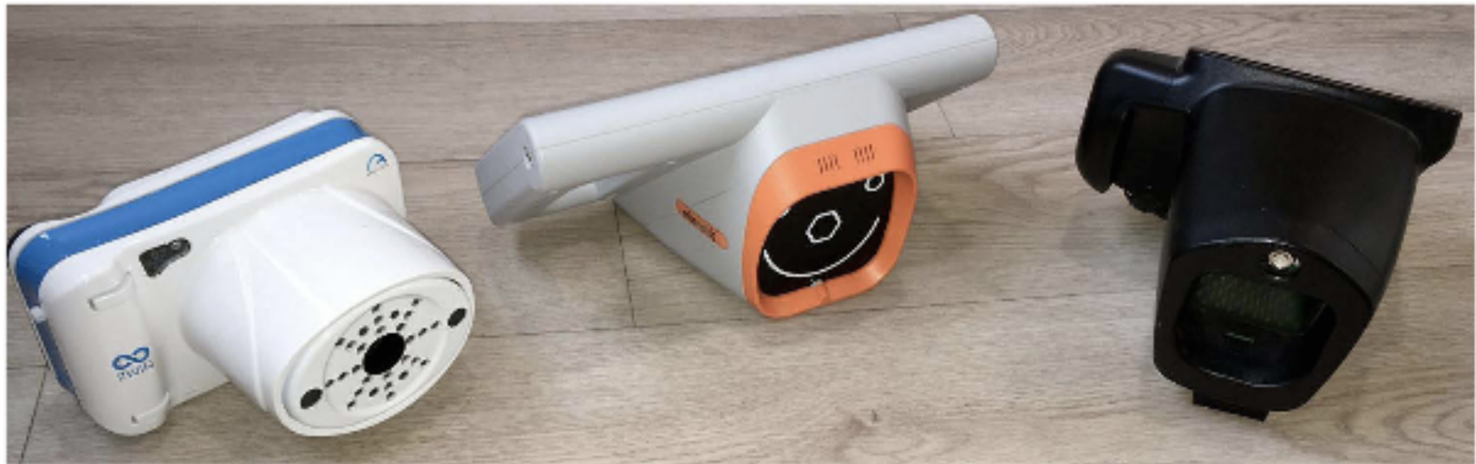
Figure 2 The three leading infrared multiradial photoscreening autorefractors; Adaptica 2WIN (left), Plusoptix A12 (center) and the Welch Allyn SPOT (right).
